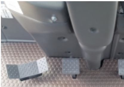
Left foot operated swing pedal avoids tiredness
